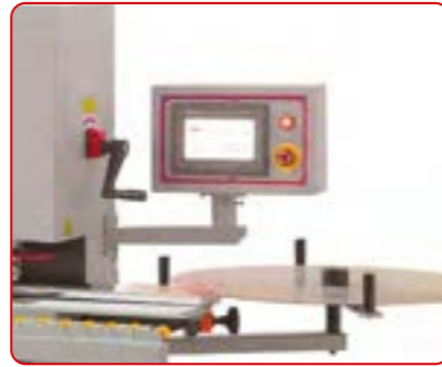
Klebetemperatur elektronisch am Touchscreen Display einstellbar gluing temperature can be set electronically on the touchscreen display
