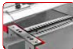
4-Messersäge inkl. Feinjustiersystem 4-knife cutterblock incl. fine adjustment
